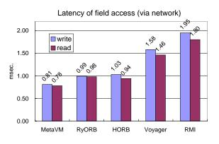
Figure 5: Latency of remote field access (two computers)
