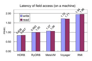
Figure 4: Latency of remote field access (one computer)
